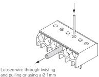
and pulling or using a  $\emptyset$  1mm release tool
