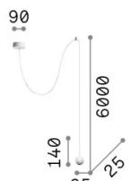
Net weight 0.16 kg Insulation class Ш **Protection index** IP20 Compliance CE **Operating temperature**
