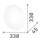
Net weight0.5 kgInsulation classIIProtection indexIP20ComplianceCEOperating temperature $0^{\circ} \sim +40 \,^{\circ}\text{C}$
