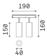
Net weight $0.33 \, kg$ Insulation classIIIProtection indexIP20ComplianceCEOperating temperature $0^{\circ} \sim +40 \, ^{\circ} C$
