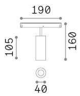
Net weight0.3 kgInsulation classIIIProtection indexIP20ComplianceCEOperating temperature $0^{\circ} \sim +40 \, ^{\circ}\text{C}$
