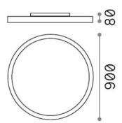
Net weight 13 kg Insulation class Ī **Protection index** IP40 Compliance CE
