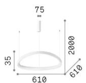
Net weight1.71 kgInsulation classIIProtection indexIP20ComplianceCEOperating temperature $0^{\circ} \sim +40^{\circ}$ C
