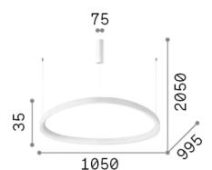
Net weight3.1 kgInsulation classIIProtection indexIP20ComplianceCEOperating temperature $0^{\circ} \sim +40 \, ^{\circ}\text{C}$
