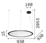
Net weight5.4 kgInsulation classIProtection indexIP20ComplianceCEOperating temperature $0^{\circ} \sim +40 \, ^{\circ}\text{C}$
