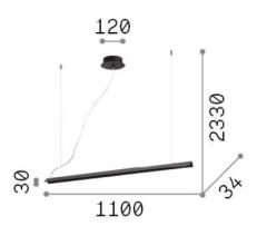
Net weight 1.14 kg Insulation class Ш **Protection index** IP20 Compliance CE Operating temperature 0° ~ +40 °C
